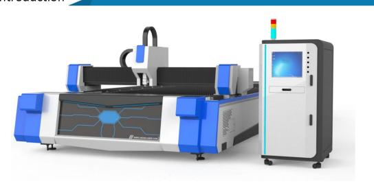
SF3015G3 fiber laser cutter reaches the top level in China, which is customers' best choice in metal industry. The bed is welded by precise welding process after annealing and aging treatment, and the beam is airborne aluminum castings. For the more, the thickness of the bed steel plate is 12 mm and the running speed can reach 100 m/min.
